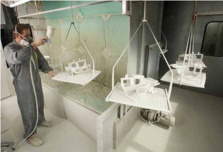
OBOVE Painting line with two spray booths incl. 240 running meters overhead conveyor
