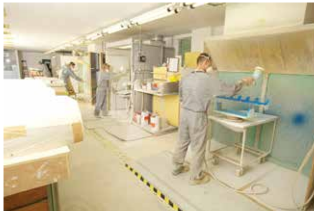
OBOVE Painting line with two spray booths incl. 240 running meters overhead conveyor
